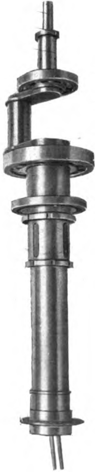
FIG. 18.—“Gnome” Engine Crank Shaft, the Oil Pipes are shown in Position.
