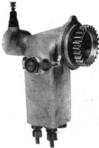
FIG. 28.—“Gnome” Lubricating Pump. This Pump and the Magneto are driven from the same Spur Wheel.
