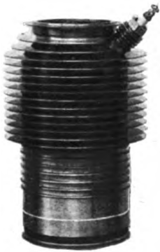
FIG. 13.—“Gnome” Engine Cylinder, showing the Groove into which the Locking Ring Fits.
