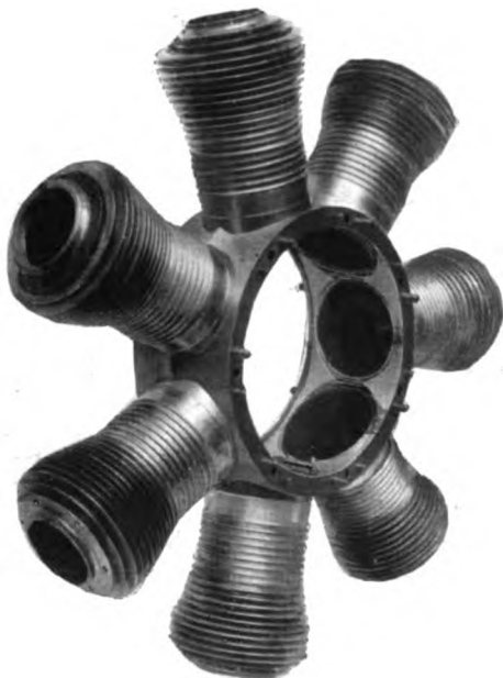
FIG. 15.—“Gnome” Engine, showing Method of Attaching the Cylinders to the Crank Chamber.
