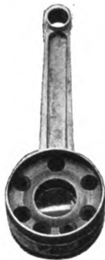
FIG. 20.—“Gnome” Main Connecting Rod, showing Holes for Subsidiary Pins.
