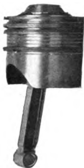
FIG. 19.—“Gnome” Piston and Short Connecting Rod.
