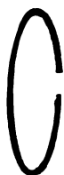
FIG. 16. “Gnome” Engine Cylinder Locking Ring. This Ring fits on the Groove round the outside of the Cylinder Trunk when inserted into the Crank Chamber.
