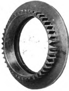
FIG. 29.—“Gnome” Spur Wheel driving the Lubricating Pump and the Magneto.
