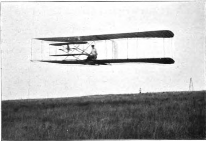
FIG. 87.—Mr Ogilvie in Flight on his Glider, notice the Gauchissement . The Starting Pylon is seen in the Distance.
