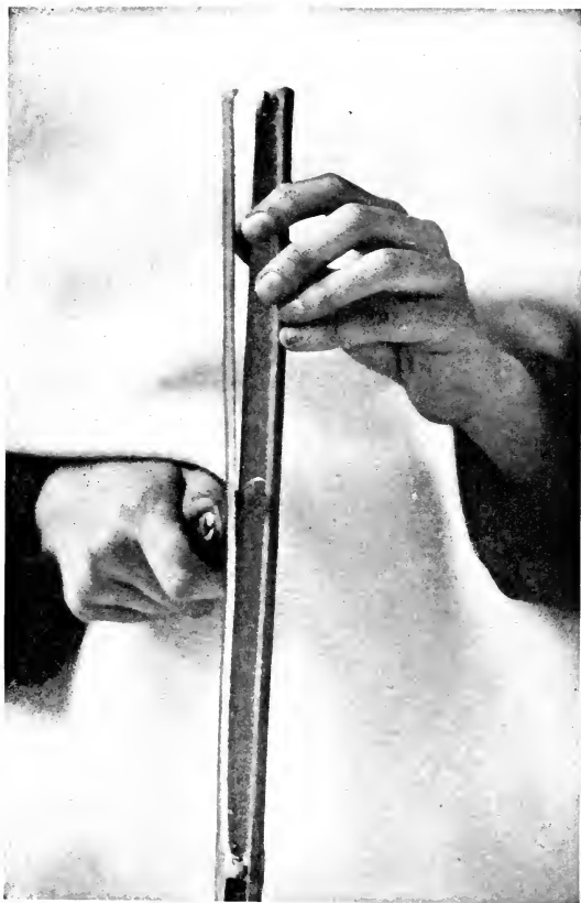
Splitting a Bamboo Fish-Pole.
