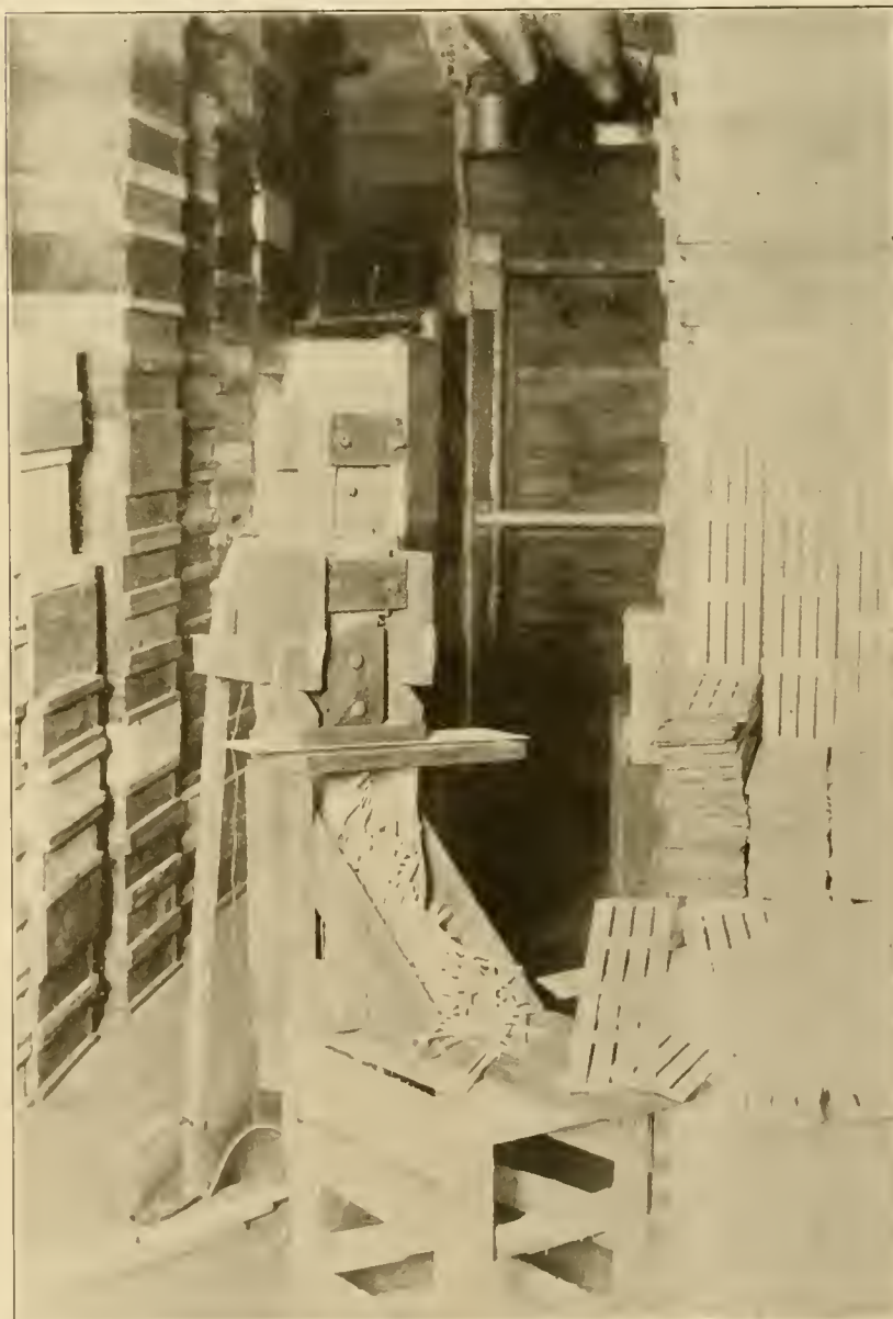
D. G. LITTLE'S HOME-MADE MACHINE FOR CUTTING SEPARATORS.
