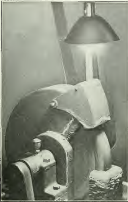
Fig. 2—Correct Lighting of an Emery Wheel
