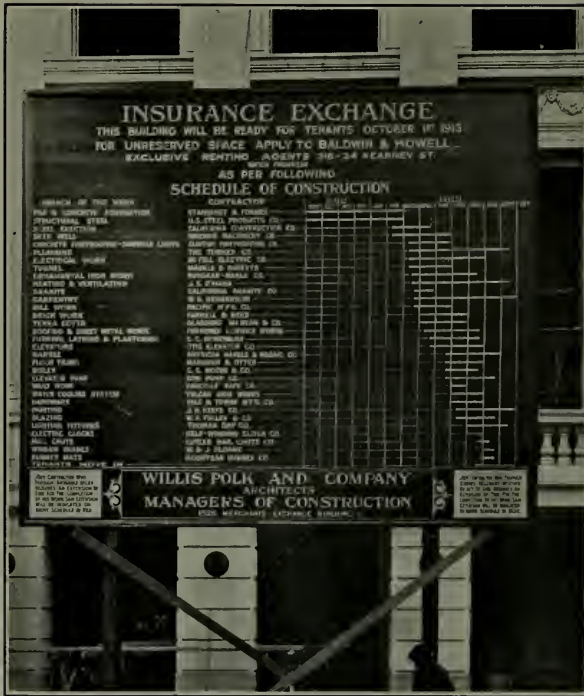
Unique Blackboard upon which was Noted the Progress Made by Each Contractor
