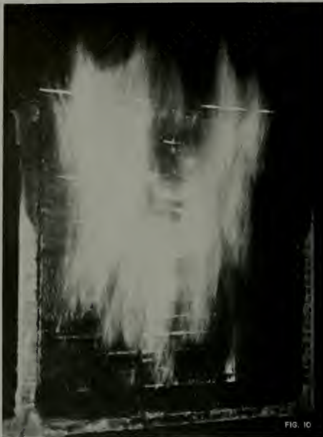
FIRE TESTS OF VERTICAL PANELS OF RED OAK—NOT TREATED EXPOSED FACE WHEN WITHDRAWN FROM FURNACE
