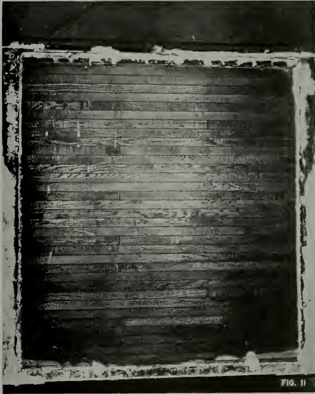
FIRE TESTS OF VERTICAL PANELS OF RED OAK—TREATED EXPOSED FACE WHEN WITHDRAWN FROM FURNACE
