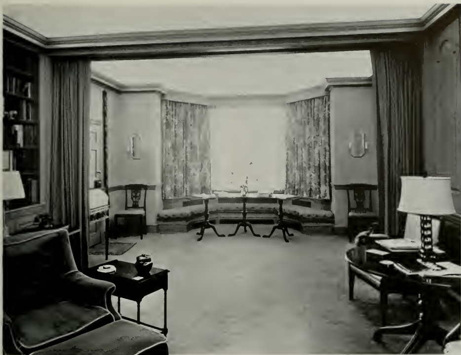
Fig. 6—A CONTINUOUS COVE OF DAYLIGHT FLUORESCENT LAMPS ILLUMINATE THIS LIBRARY AND SUN-ROOM
