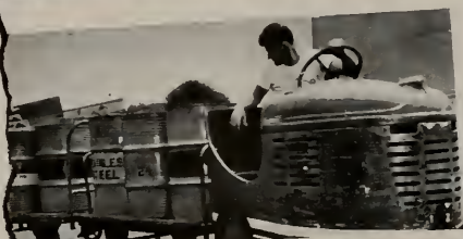
SEGREGATION MINIMIZES SCRAP LOSS - A western aircraft plant has more than doubled its scrap collections through a systematic salvage program, directed from a central office. All metal scrap is segregated into solids and machining, and also by alloy content, right at the machines. Scrap containers are color-banded and labeled to clearly identify what goes into each. . . . Have you organized an efficient scrap collection system at your plant? Does it provide for careful segregation?
