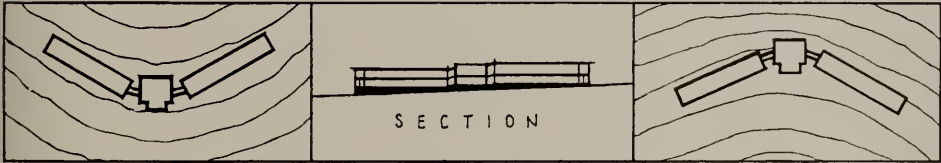
PLAN DIAGRAM SHOWING HOW BUILDING GROUPS CONFORM TO GRADES
