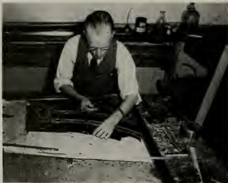
This is a picture of Mr. Walter Swatfield shown glazing one of the sections of a large window. The lead extrusions are being cut and the pieces fitted into their respective positions, later the joints will be soldered.
