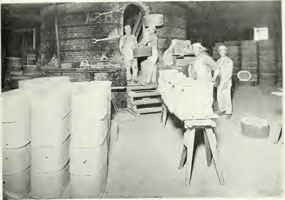
Loading a kiln. Suggers are shown piled at side. All pieces are enclosed in these during firing.
