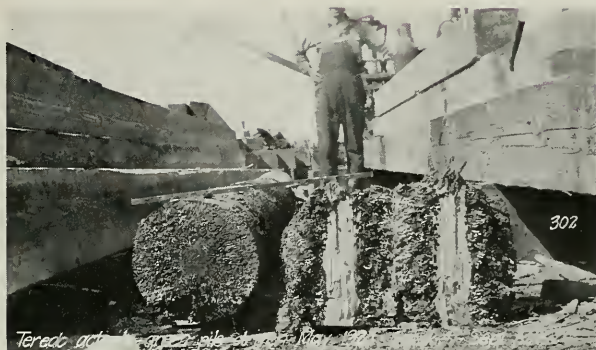
WHAT THE TEREDO ACCOMPLISHED IN TWO MONTHS AT CROCKETT, CAL. Wooden pile driven May, 1924, and pulled September 19, 1924. First attack of Teredo on July 15. Pile 12 inches in diameter completely riddled by Teredo at the mud-line shown in split sections. Courtesy of Prof. C. Derleth.
