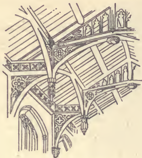
Hammer Beam Roof
