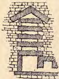
FIG. 2. Corbelling over King's Chamber.
