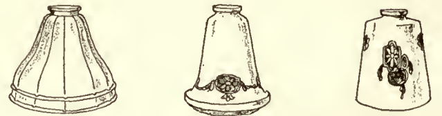
Types of Direct Lighting Reflectors
