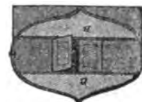
Fig. 11.—B, Water-tight Bulkheads, Sections at end of Midship Sections, showing the sections as a Deck-house.
