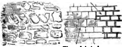
Rubble Fine Jointed
