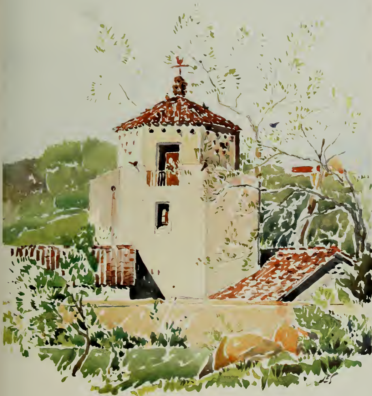
“THE DOVECOTE” of the Farm Group on the Thomas Ince Estate, Beverly Hills. Roy Seldon Price, Architect . The roof is random laid with Varicolored Granada tile made by Gladding, McBean & Company—Los Angeles Pressed Brick Company. Watercolor sketch by J. E. Stanton.
