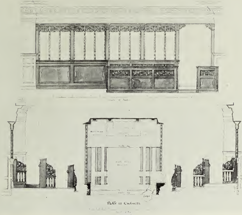
PLATE CII.—S. BOTOLPH'S, ALDGATE: CHANCEL SEATS AND SCREENS OF OAK.
