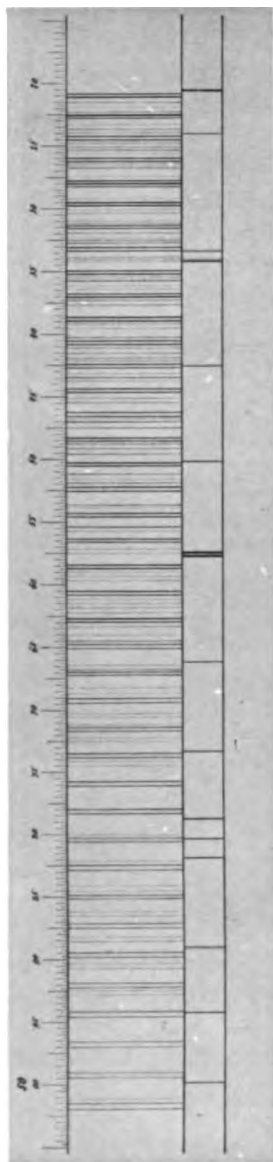
The Spectrum of Aluminium Oxide as Photographed by Professor B. Hasselberg.
