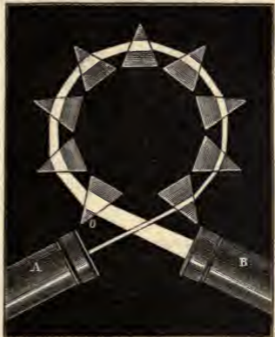
Fig. 17.—Spectroscope, with Battery of Prisms.
