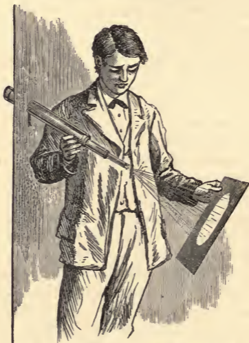
Fig. 37.—Holding Telescope to see the Sun's Spots.
