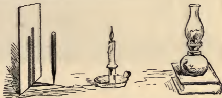
Fig. 8.—Measuring Intensities of Lights.
