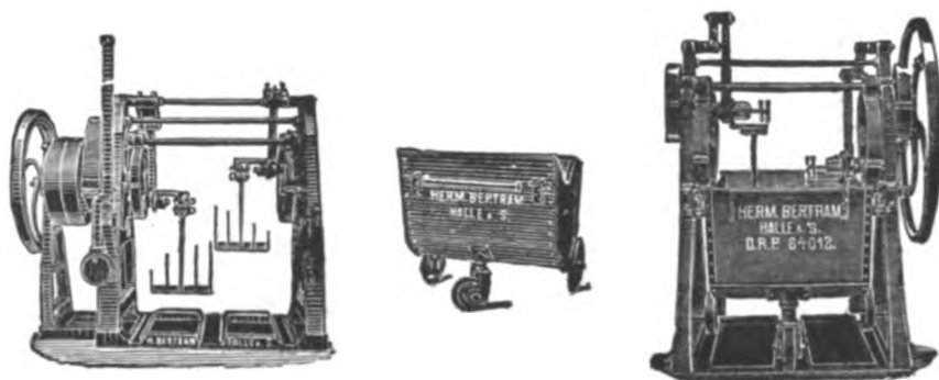
Fig. 235.—Dough Mixer of H. Bertram (Removable Trough).
