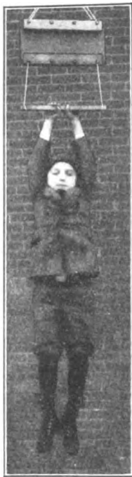
A sheet of Three-ply AIRCO (between clamps) holds up a 68-pd. boy.
