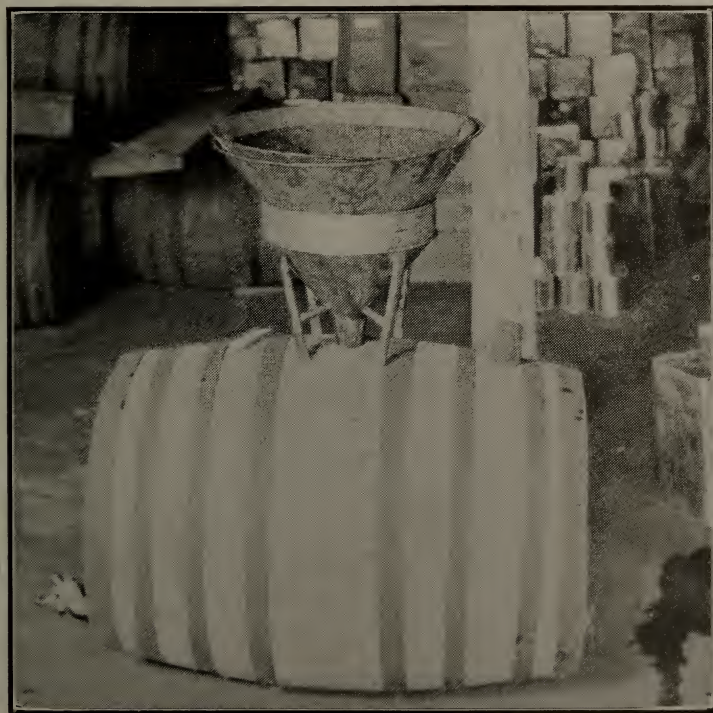
Fig. 24. The Dadant strainer for barrels.
