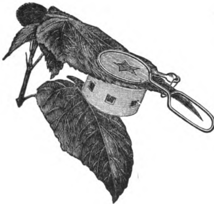
FIG. 3.—A light screen for experiments in starch formation by leaves; \times \frac{1}{2} .
