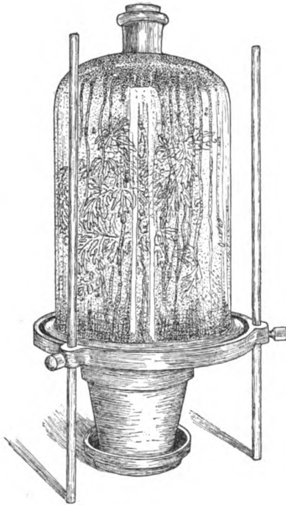
FIG. 18. — A conclusive demonstration of transpiration; \times \frac{1}{2} . The bell jar was dry when placed over the plant. Its bottom is a plate split and perforated in such a way as to fit closely around the stem of the plant.
