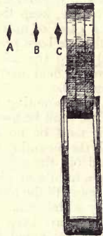
FIG. 86.—Diagram illustrating how to focus a hand-lens. A, the distance of the object from the lens when in focus with the low power; B, with medium; and C, with high power.
