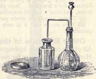
FIG. 145.—Diagram of apparatus for the preparation of carbon dioxide.
