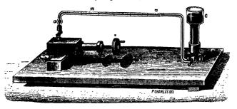
Fig. 8.—Apparatus of Bonnier and Mangin, for analysis of gases given off by plants. c, Reservoir of Mercury; m m, graduated tube; n, screw of piston, which enables the gas to be drawn into the graduated tube and measured; and after it the potash and pyrogallic solutions successively, each being thoroughly brought into contact with the gas in the dilatation a.
