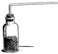
FIG. 2. — Soaked Peas in Stoppered Bottle, ready for Exhaustion of Air.
