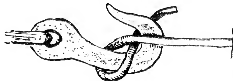
Becket hitch, for joining a cord and a rope.
