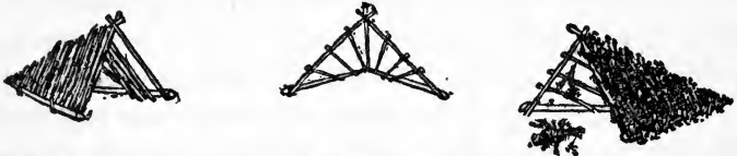
How to Build and Thatch a Brush Shelter After the Plan of the Old Indian Camp
