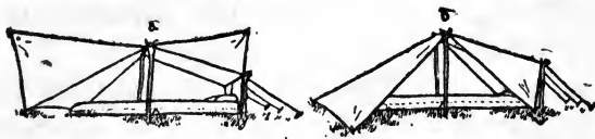
Two Views of Phillips Tent Pitched with Tick and Ridge-Pole. In a the Flaps are Up, Showing How They May Be Turned Back; b Shows Them Pegged Down for the Night
