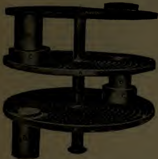
Fig. 29—Detail of Chamber, Continuous Still.
