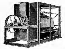
A simple mechanical Tapping Device keeps the screen clear without the employment of labor to clean out clogged materials. The ideal Tankage Screen.
