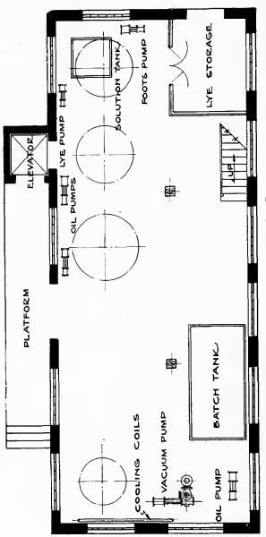
FIRST-FLOOR PLAN OF VEGETABLE OIL REFINERY
