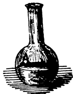
Fig. 45.—Dis- solving silver in nitric acid.
