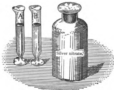
Fig. 6.—Behaviour of distilled and undistilled water with silver nitrate solution.
