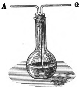
Fig. 36.—Detection of carbon dioxide in expired breath.
