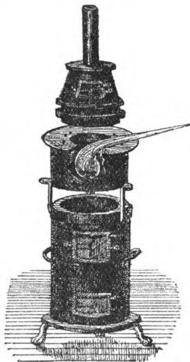
Fig. 34.—Heating tin in a closed retort in a furnace.
