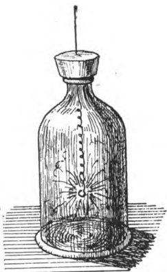
Fig. 32.—Iron burning in oxygen.
