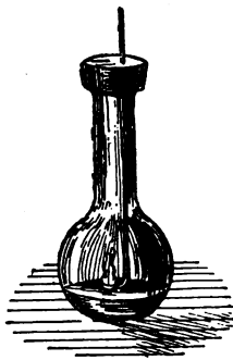
Fig. 41.—Experiment to show that an acid is formed by burning sulphur.
