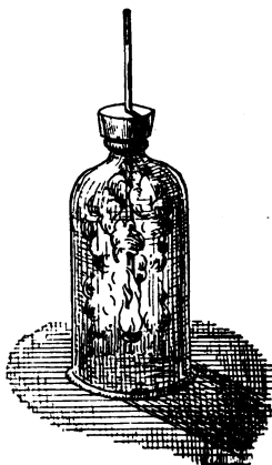
Fig. 31—Phosphorus burning in oxygen.
