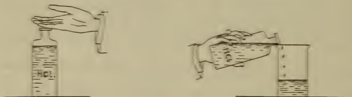
Method of Handling Reagent Bottles
