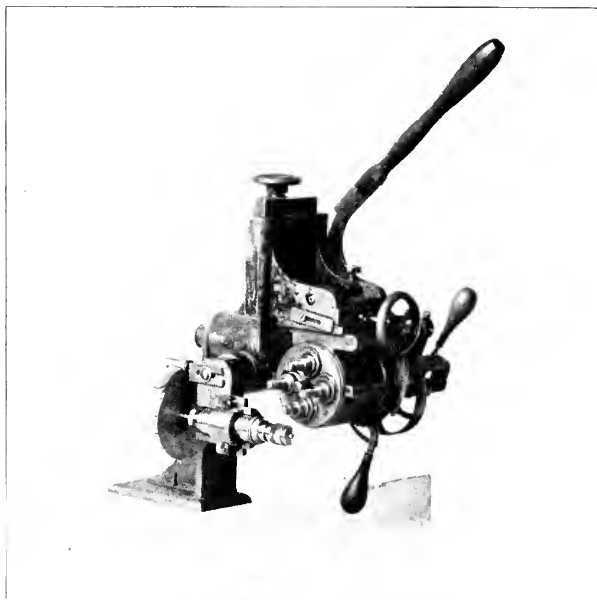
Fig. 28.—Old Escape Wheel Cutter.
