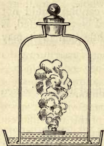
FIG. 5.—Apparatus for finding the amounts of oxygen and nitrogen in air.
