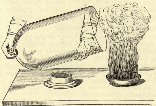
FIG. 14.—Extinguishing a burning liquid by using a vessel full of carbon dioxide.
