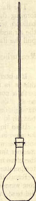
FIG. 42. — Flask fitted ready for filling with water ; to show expansion on warming.
