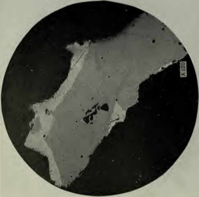
A. TETRADYMITÉ (WHITE) AS A PARTIAL RIM ON BISMUTHINITE (GRAY) BETWEEN QUARTZ CRYSTALS (BLACK).
