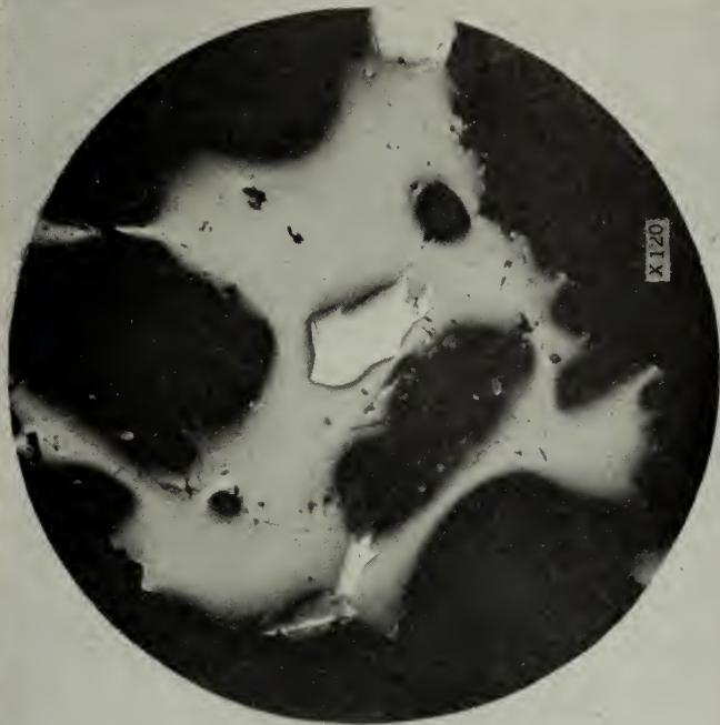
B. GOLD (WHITE) IN GALENOBISMUTITE (GRAY) AS A FILLING BETWEEN QUARTZ CRYSTALS (BLACK).
