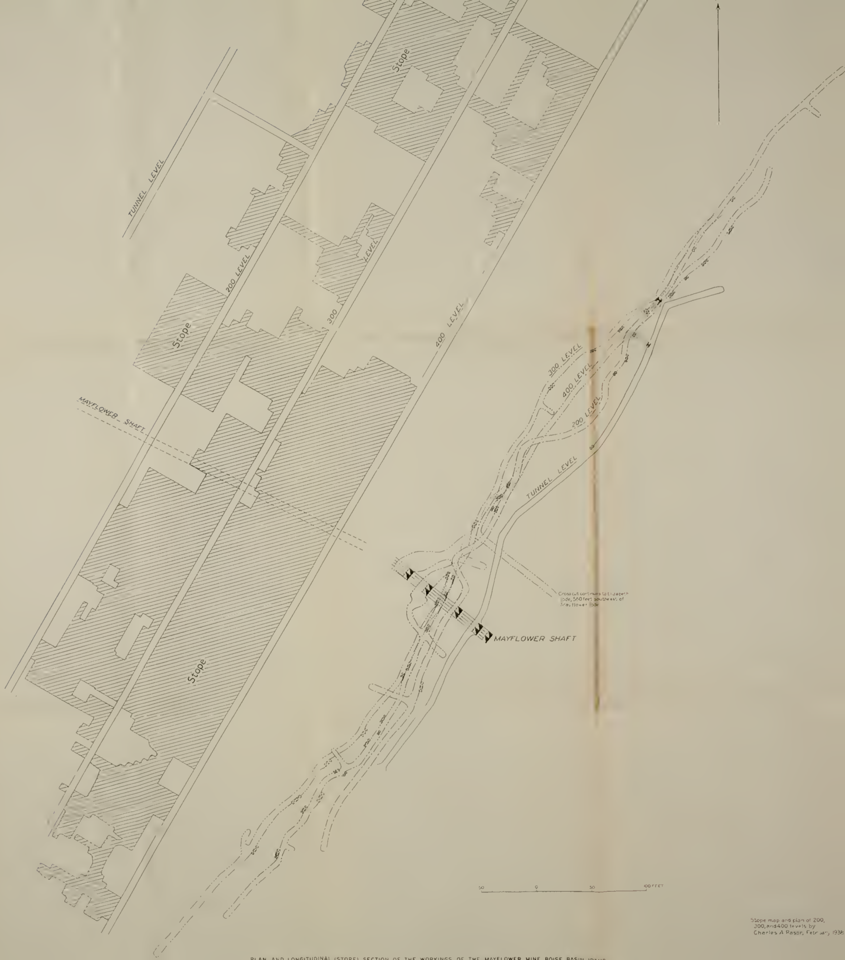
PLAN AND LONGITUDINAL (STOPE) SECTION OF THE WORKINGS OF THE MAYFLOWER MINE, BOISE BASIN, IDAHO
