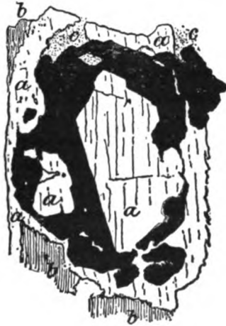
Fig. 7. Primary pyrrhotite in augite. Black, pyrrhotite; a, augite; b, uranite;† c, chlorite. From W. Lindgren; 17th Annual Report United States Geological Survey, Part II.
