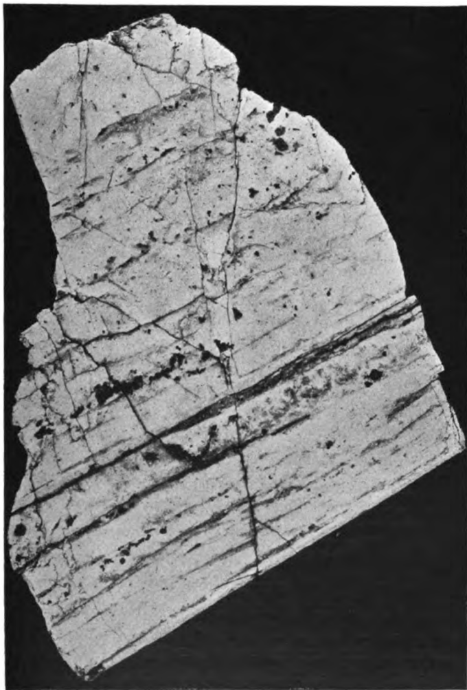
Fig. 48. Vein quartz, showing ribbon structure; from Providence mine, Grass Valley district, California. After Waldemar Lindgren.*
