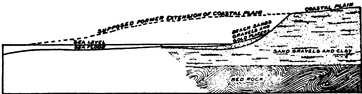
Fig. 56. Diagrammatic section of beach placers at Nome, Alaska. After Schrader and Brooks.*
