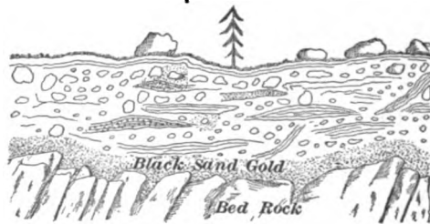
FIG. 105.—PLACER BED SHOWING LOCATION OF "BLACK SAND" ON BEDROCK.
