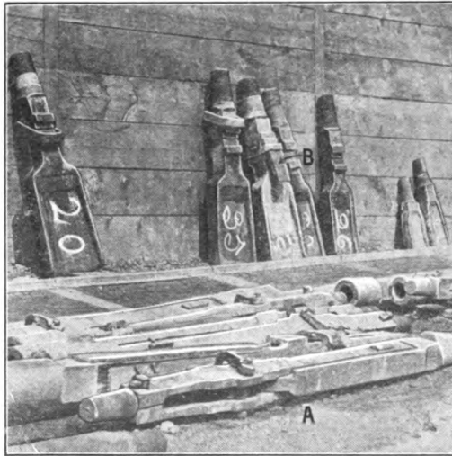
FIG. 51.—Boring Tools used at Easington Colliery Sinking, Co. Durham, in 1903.
