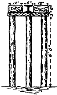
FIG. 119.—Mode of supporting the Roof at the Delivery End of a Conveyor.
