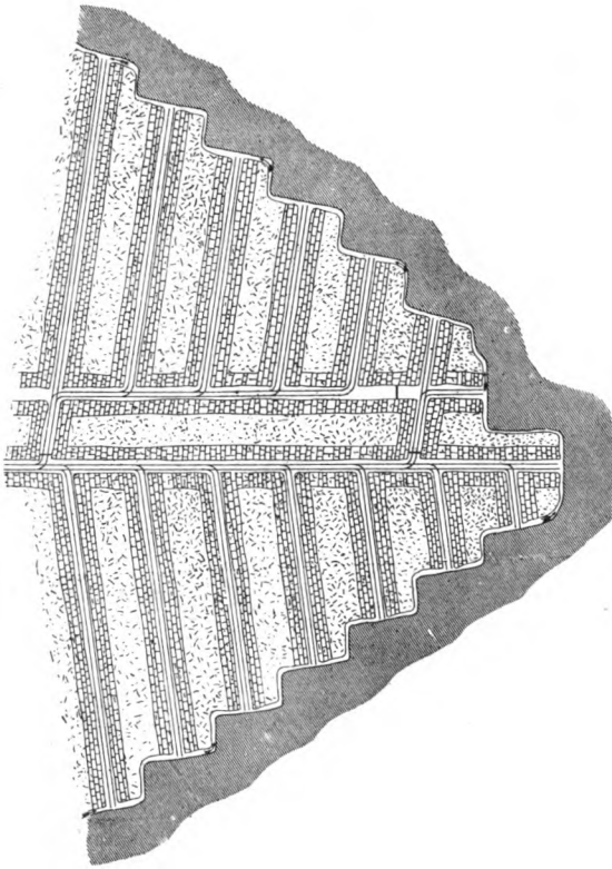
FIG. 113.—Long-wall Workings in a Thin Seam, the Roadways being maintained through the Goaf.
