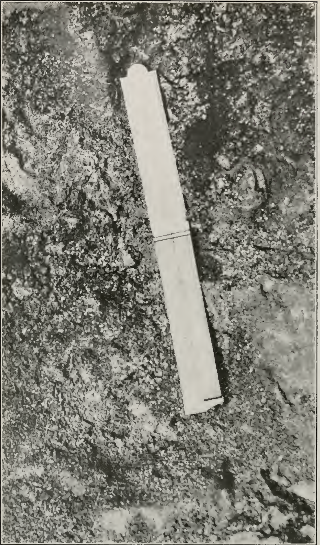
Photo No. 50. Quicksilver in earth and gravel under site of old furnaces at New Almaden. The numerous 'white' spots are globules of quicksilver.
