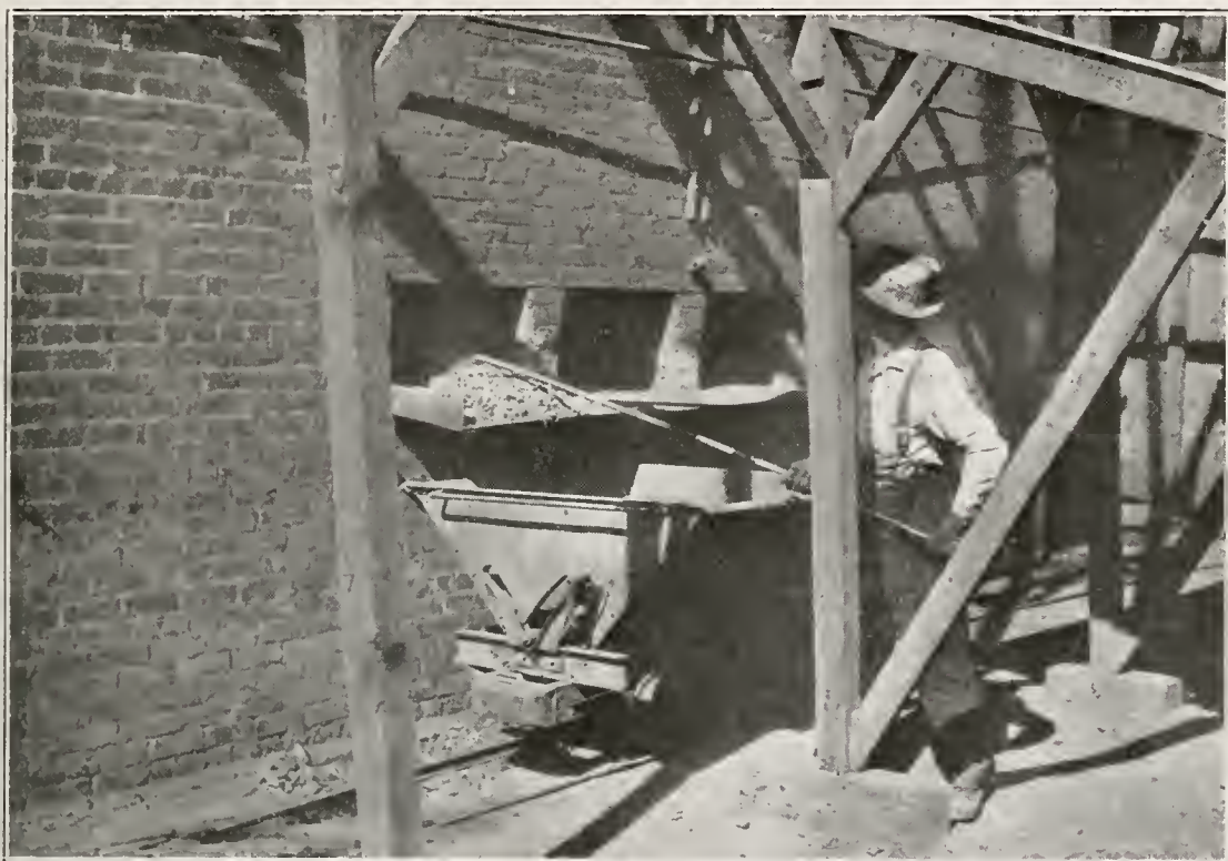
Photo No. 4. Drawing off burned ore, New Mercy (Pacific) Quicksilver Mine, Fresno County.
