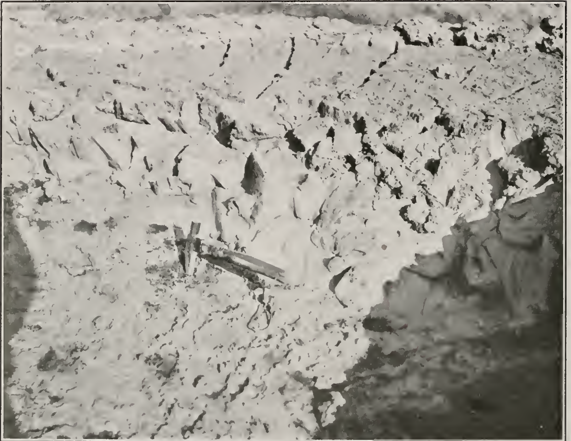
Photo No. 76. Flotation Concentrates drying in the sun, at the Senator Mine of New Almaden Company, Santa Clara County.
