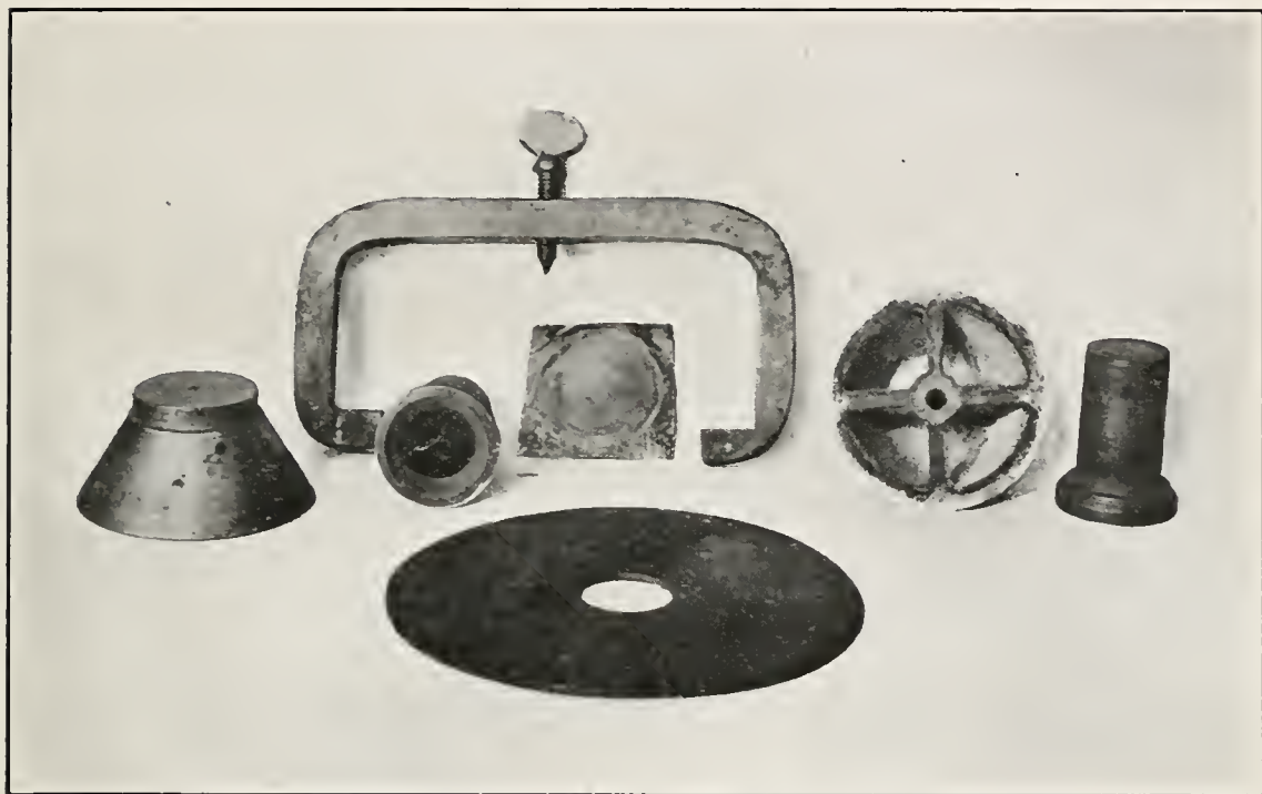
Photo No. 68. Whitton Quicksilver-assay Apparatus, showing component parts.
