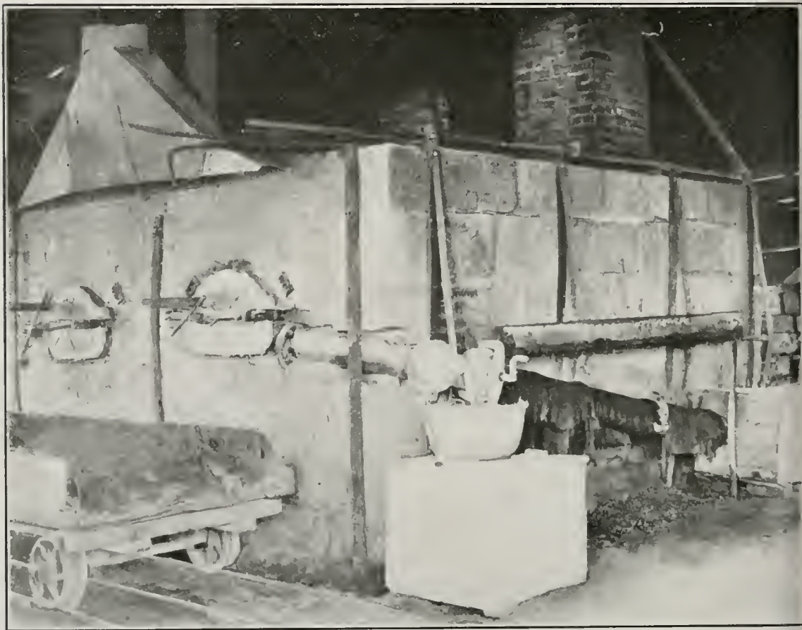
Photo No. 41. 'D' retorts at Aetna Mine, Napa County. The 'T' of 1" pipe at retort door is the inlet for air circulation. Water-wheel and fan are at right, just out of picture.
