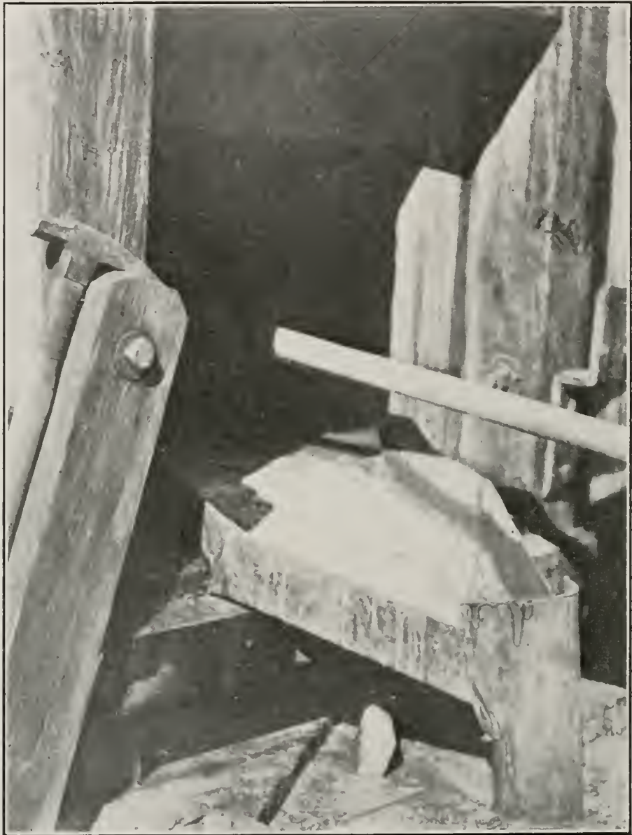
Photo No. 66. Cleaning up one of the new, wooden condensers at New Idria. The bright globules of metallic quicksilver and the 'gray mud' may be seen on the discharge lip.
