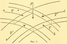
a, b, and c, d, at right angles to each other, and of unit breadth; T the tangential thrust on any of the faces of the unit square, respectively opposite (which, as being small in relation to the radii of curvature, may be considered as plane).
