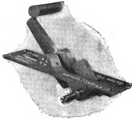
FIGS. 1115 AND 1116.—HOLLINGS' PATENT TUB STOPPER.
