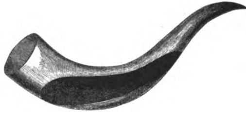
HORN, SHOWING METHOD OF CUTTING SPOON.
