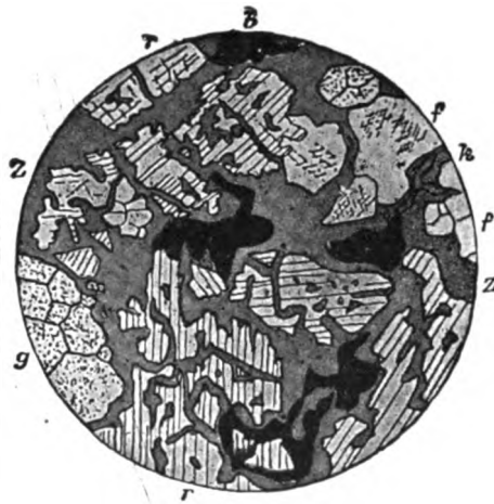
Fig. 200.—Garnet-rhodonite aggregate with immigrated ores. (Enlarged 50 times.) g, garnet; r, rhodonite; f, fluorite; b, galenite; z, blende; k, chalcopyrite.
