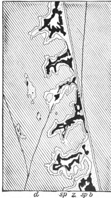
Fig. 231.—Ore deposit of the Josefi-Blatt, near Nordfeldort, Aloisi adit. (Posepny.) d, dolomite; z, sphalerite; b, galena; sp, magnesian spar.
