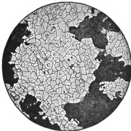
Fig. 190.—Limestone (c) replaced by galena (g), prite (p) and secondary quartz (q). Elkhorn Mine, Montana. (Enlarged 12 times.)
