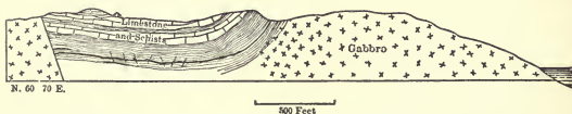
FIG. 47.—Cross-section of the Cheever iron mine, near Port Henry, N. Y., showing the occurrence of the ore in pyroxene gneiss, just over gabbro. Lake Champlain terminates the section at the right. After J. F. Kemp, Bull. N. Y. State Museum , Vol. III, p. 346.
