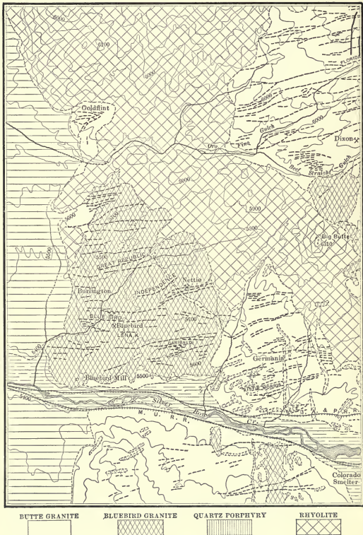
FIG. 58.—Geological map of the Western half of Butte District, Montana, reproduced in line-work from the colored map of the Butte Special Folio, U. S. Geological Survey.
