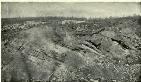
FIG. 21.—View in Cherry Valley Mine, showing sandstone with underlying cherty clay. The sandstone dips southeast inward toward the ores. After F. L. Nason, Report on Iron Ores of Missouri, p. 125. Plate VI.
