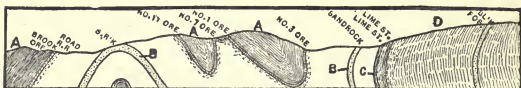
FIG. 11.—Geological Section of the Low Moor, Va., Iron-ore Bed. After B. S. Lynn, Trans. Amer. Inst. Min. Eng. , XIV., 801. A—Marcellus Shale; B—Oriskany Sandstone; C—Lower Helderberg Limestone; D—Clinton Shales.
