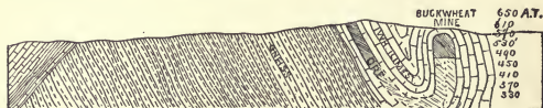
FIG. 84.—Cross section at Franklin Furnace, N. J., corresponding to AA. of map (FIG. 88), and four times the scale of map. At the left is blue limestone and quartzite. After J. F. Kemp, Trans. N. Y. Acad. of Sciences , XIII., 86, 1893.
