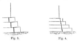
cross strain thrown on the projecting portion of the masonry will rend it from top to bottom, as shown in Fig. 4.
