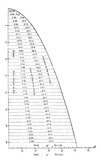
force of the blow given by a ram whose weight = 1, with falls varying from 1 to 40 ft., can be at once read off by inspection. (See previous page.) Thus the momentum of a ram weighing 1 ton and
