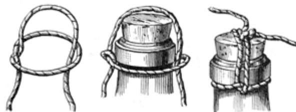
METHOD OF TYING DOWN CORKS IN KOUMISS BOTTLES.
