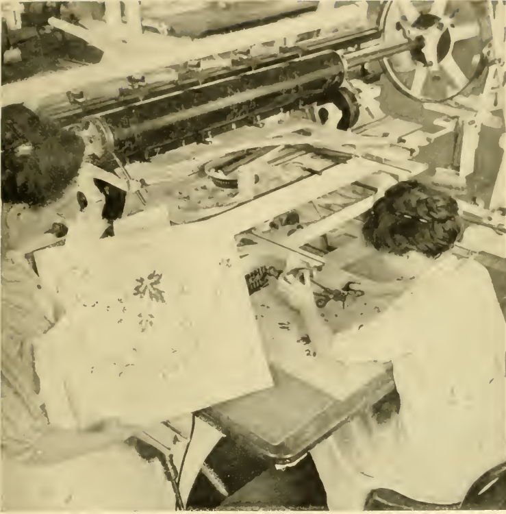
Transferring Design to Copper Roller.
