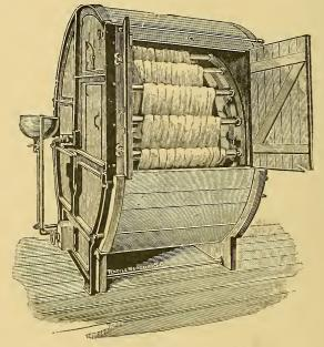
Fig. 52.—Hank and Slubbing Dyeing Machine.
