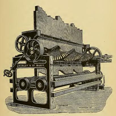
Fig. 73.—Beetling Machine.
