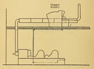
Fig. 2.—Hopper Feeder (in upper room) applied to Opener (on ground floor).
