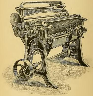
Fig. 10.-Card-Grinding Machine.
