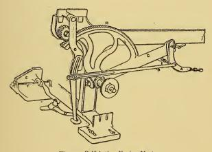
Fig. 22.—Self-Acting Nosing Motion.
