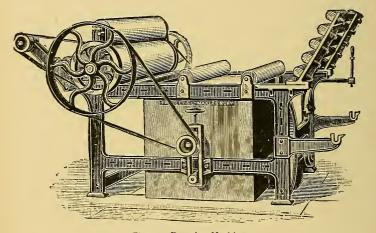
Fig. 43.-Damping Machine.
