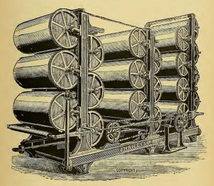
Fig. 40.-Vertical Drying Machine.
