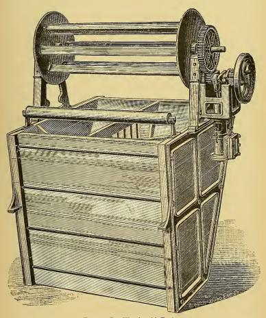
Fig. 50.—Dye Wench, with Engine.
