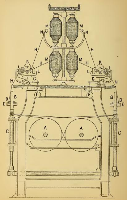
Fig. 26.—Ring Spinning Frame.
