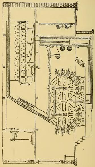
Fig. 54.-Eight-Colour Duplex Calico Printing Machine.
